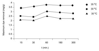
Fig. 4. Effect of temperature on the removal of Tar-Chromium Green 3G by diatomite (conditions:  $C_o 5 \text{ mg/cm}^3$ , natural pH, adsorbent 3.0 g, t = 15 - 300 min)
