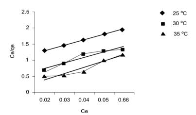
Fig. 6. Langmuir isotherms of the dyes adsorption onto diatomite at different temperatures
